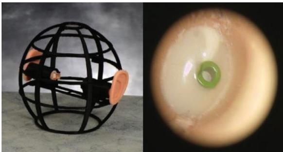
**Figure 1.** Image of modular Tympanostomy tube simulator.
